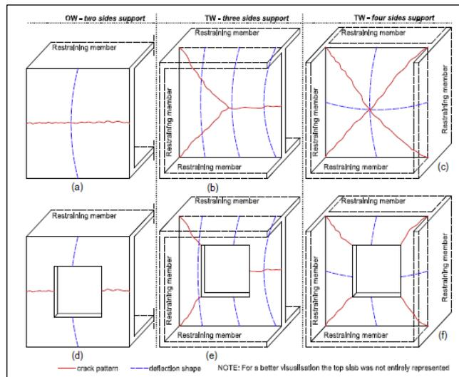
**Figure 2.** Typical crack pattern and deflection shape of axially loaded reinforced concrete walls (Popescu et al., 2015b)
