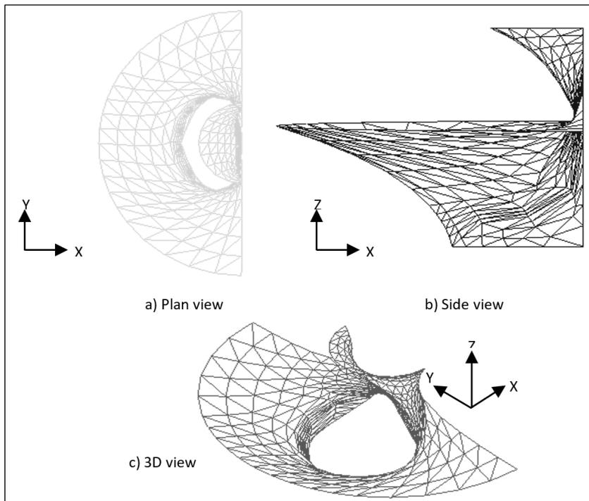
Figure 11. Different Views of Half-Costa Tensioned Membrane Structure model in XZ-Plane after Form-Finding (with larger opening)
