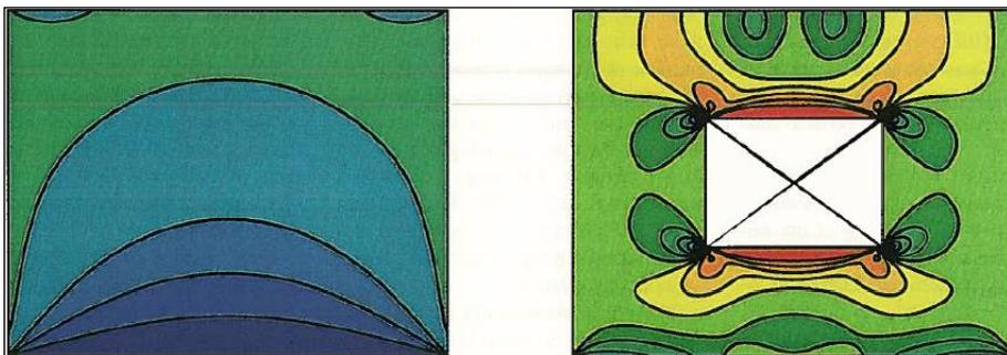
**Figure 3.** Stress contours in the wall panel with opening and without opening (Michael et al., 2002)
