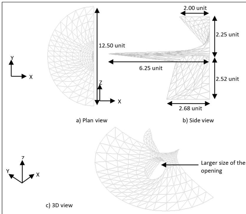
Figure 10. Initially Assumed Shape of Half-Costa Tensioned Membrane Structure model in XZ-Plane (with larger size opening)
