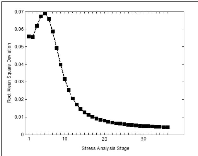
Figure 13. Variation of RMSD versus Stress Analysis Stage of Half-Costa Tensioned Membrane Structure Model in XZ-Plane (with larger size opening)
