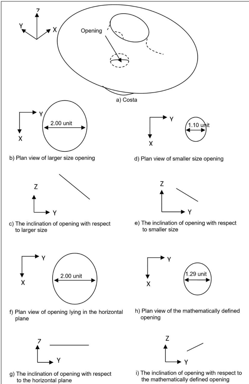
**Figure 9.** Initially Assumed Shape of the Opening in Half-Costa Tensioned Membrane Structure Model in YZ-plane
