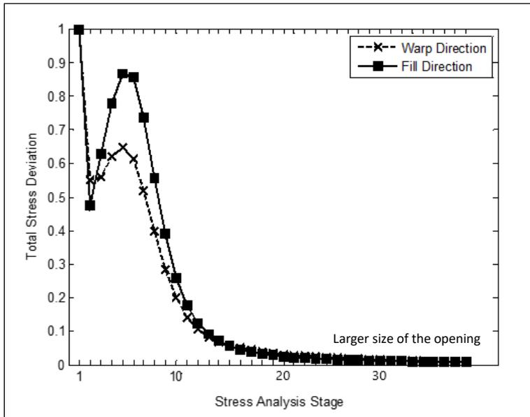
Figure 12. Variation of Total Stress Deviation in Warp and Fill Direction versus Stress Analysis Stage of Half-Costa Tensioned Membrane Structure model in XZ-Plane (with larger opening)
