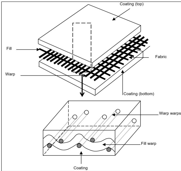
Figure 6. A basic structure of the coated fabric
