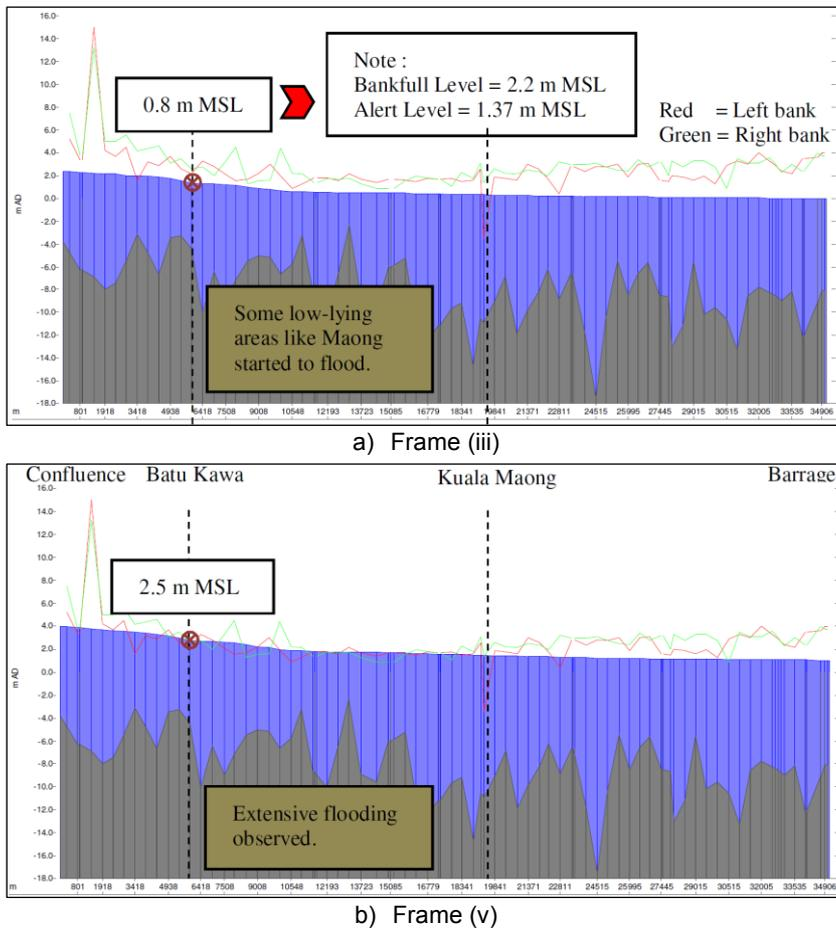
Figure 8. Long section profiles of Sarawak River for January 2004 flood event
