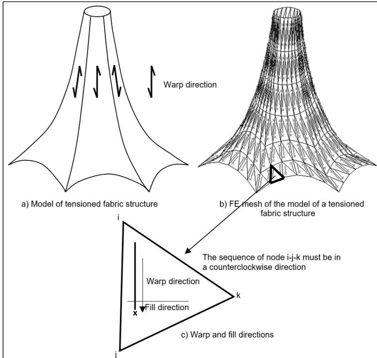
Figure 7. Meshing and element node sequence
