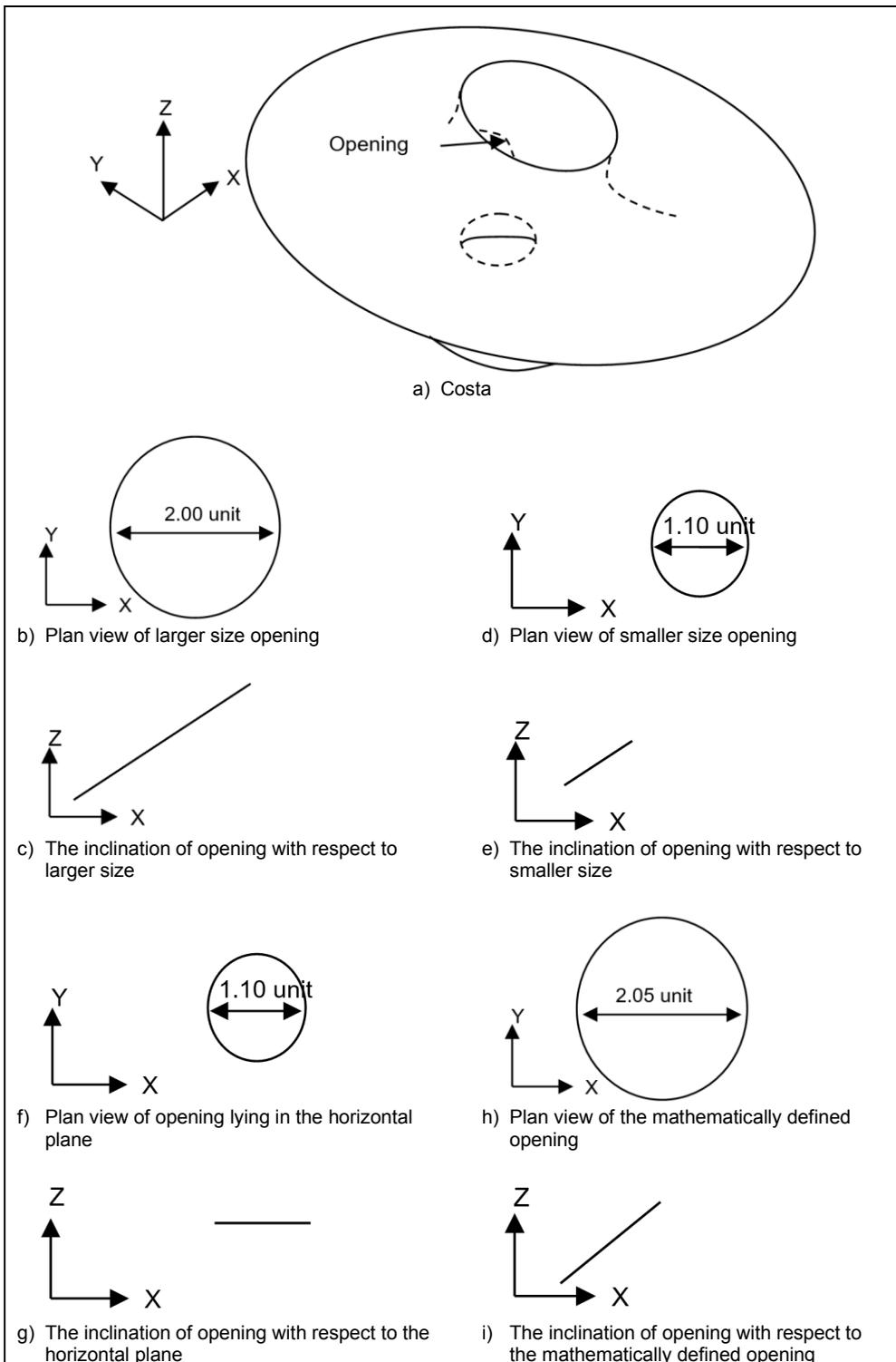
**Figure 8.** Initially Assumed Shape of the Opening in Half-Costa Tensioned Membrane Structure Model in XZ-plane
