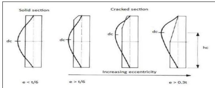
Figure 4. Effect of increasing eccentricity on the size of cracked section small (Kuddus, 2010)
