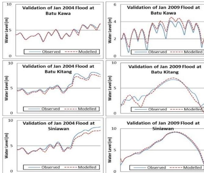
**Figure 3.** Model calibration of January 2004 and January 2009 flood events at Batu Kawa, Batu Kitang and Siniawan
