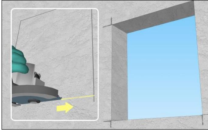
**Figure 1.** Cut out opening for a window opening, WikiHow (2018)
