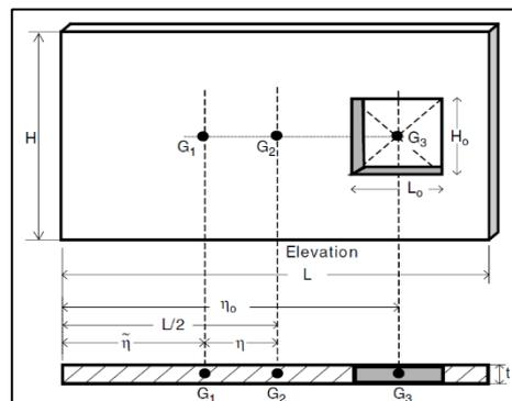
Figure 6. Definition of parameters in design equations, Saheb and Desayi (1990a)
